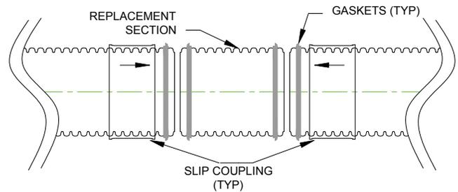
**Large Diameter Repair Coupler** 12- through 60-inch (300 – 1500 mm) are ideal for repairs and alterations of large diameter sewer pipe. Repair couplers similar to those provided by Mission Rubber Company LLC, Fernco® or equal may be used on SaniTite HP pipe.
