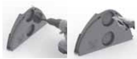
5. Place lip of end cap over the end of the chamber unit and snap into place. Secure in place with backfill. The universal end cap is designed to fit both ends of the Arc 36 and Arc 36 HC chamber. The end cap shall be placed so that the Arc logo faces outward. Receiving pockets for 6” x 8” splash plates are incorporated into every end cap.
