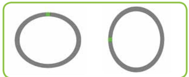
Figure 19: Pipe Rotation for Re-Installation (Deflection exaggerated for illustration)
