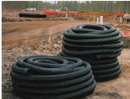
**ADS single wall corrugated pipe** serves well for localized collection and drainage. Offered in both perforated and non-perforated styles in 3" through 24" sizes.
