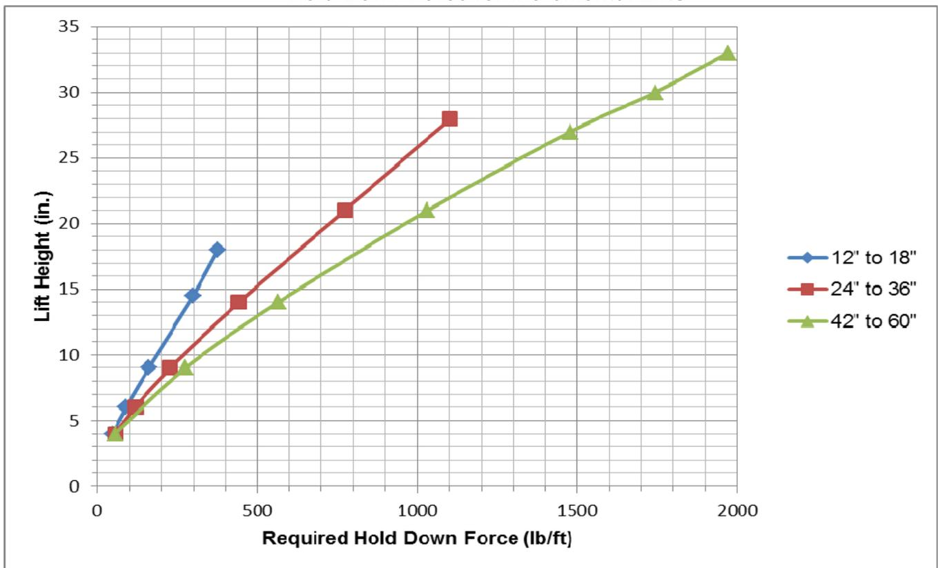
\*Assumes a unit weight of flowable fill of 150 pcf and no water in the pipe at time of placement
